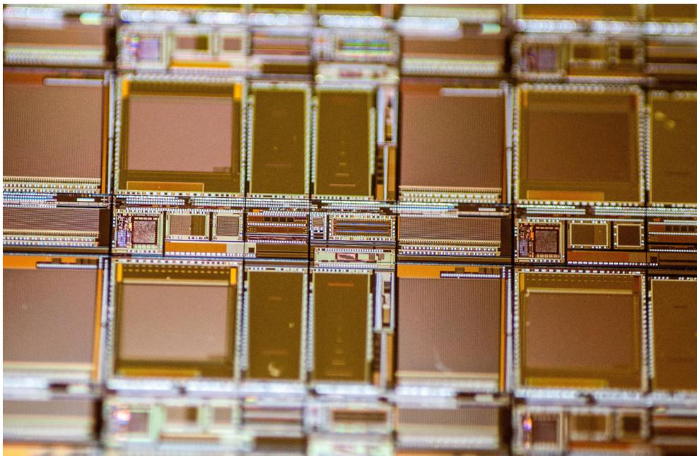
SPAD sensor chips are implemented in CMOS technology. © Fraunhofer IOSB | Picture in color and printing quality: [www.fraunhofer.de/en/press](http://www.fraunhofer.de/en/press)
